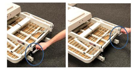
4. Near the casters are two 7/16-14" X 4 <sup>1</sup>/<sub>2</sub>" zinc bolts, these need to be removed with the 5/8" socket and drill. Retain these bolts and nuts for assembly process.
