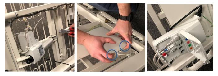
7. Plug cables 3 (Green) and 4 (Orange) into the respective locations. Route the cabling to seat into he groves of the control box and then close tightly.
