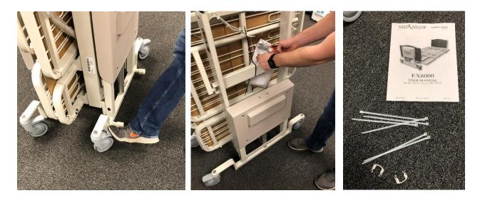
2. Lay the bed in the shipping form onto the side with the rubber bumpers.
