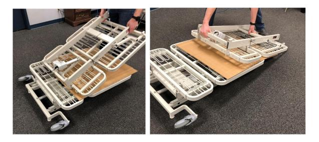
7. Unbolt the other two 7/16-14" X 4 <sup>1</sup>/<sub>2</sub>" Bolts and remove the head section assembly from the head high low assembly. Remove and retain hardware for assembly process.
