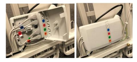
8. Return the bed to its casters. Cut all cable ties from bed in these locations. Remember to include removing the handset below the head end of bed deck.
