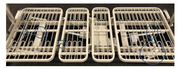
9. Plug the high low cable into actuators, use the provided c-clips to secure the cable (be sure to push in until flush with plastic housing). Route the wire along the weldment and secure with the provided cable ties. Cut off any excess cable tie.
