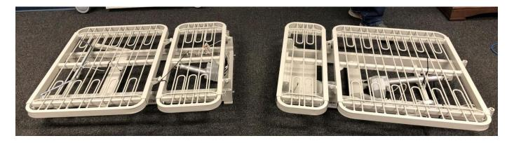
9. There are two more 7/16-14" X 1 <sup>3</sup>/<sub>4</sub>" bolts that need removed, located on the foot end deck assembly, retain hardware for assembly process.
