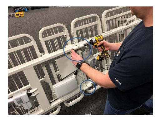
5. Use the two 7/16-14" X 1 <sup>3</sup>/<sub>4</sub>" bolts and nuts to secure the inside frame to each assembly. Be sure to use the impact drill again to firmly secure.
